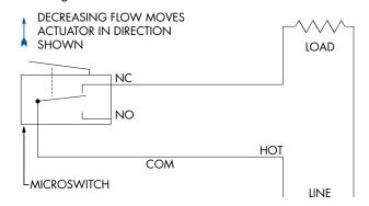
**Fig 2**: Wiring schematic for power applied to load when flow is greater than set point (power to load interrupted when flow decreases to below set point).
