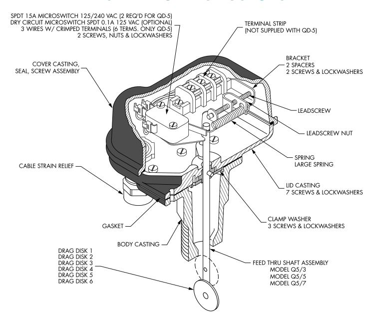
This parts list applies to all models of Q-5 and QD-5 fluid flow switches: Q-5/3, Q-5/7, QD-5/7.
